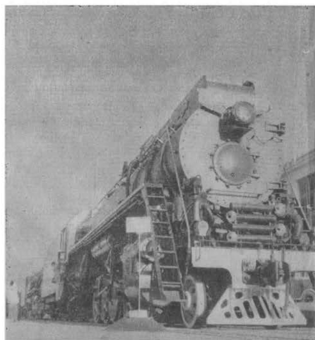
The Peace locomotive for freight trains, 3,340 h.p., designed and built in China
