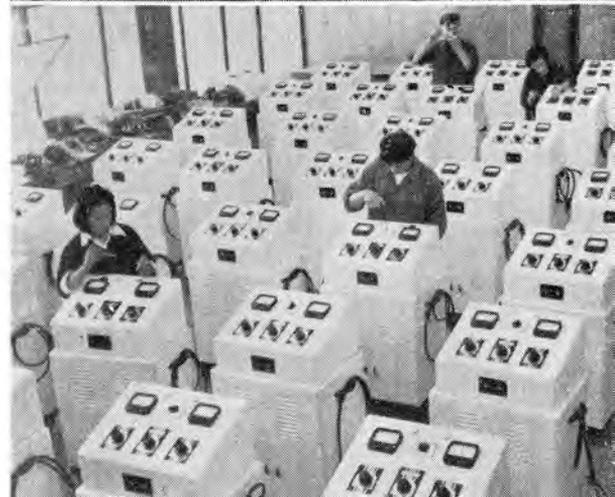
Short-wave medical apparatus, mass produced by the Shanghai State-owned Medical Precision Machinery Works
